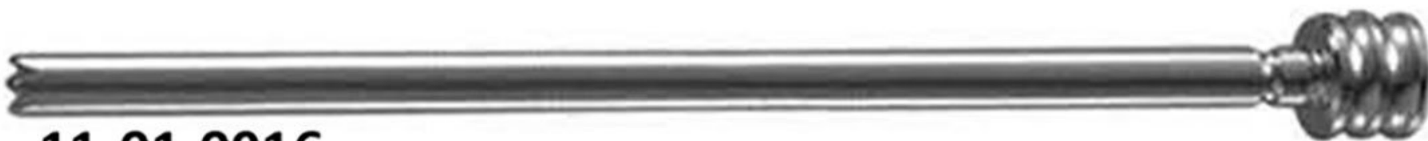
11-01-0916 Drill Sleeve 4.5/ 2.0 Length 109mm, for percutaneous insertion of 7.0mm cannulated screws
